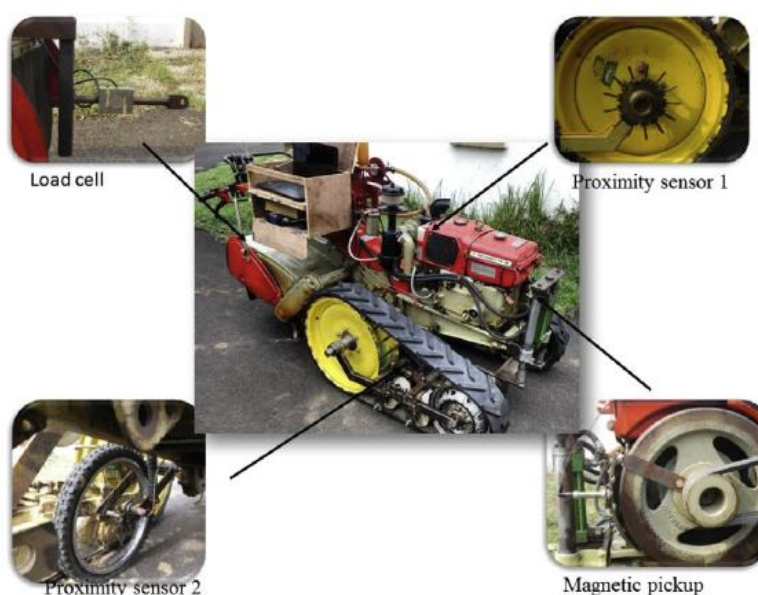
Fig. 5 – Instrumented walking tractor.
