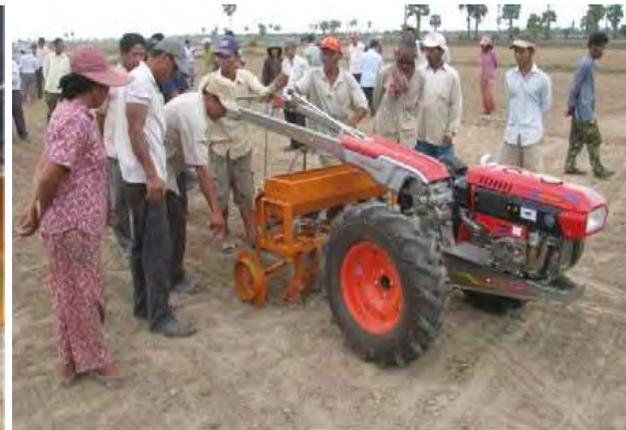
**SE-2009-037 project developed Cambodian disc and tine drill prototypes demonstrated in the provinces**
