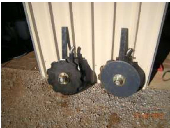
Optional staggered double disc opener (left) and cutting coulter disc (right)
