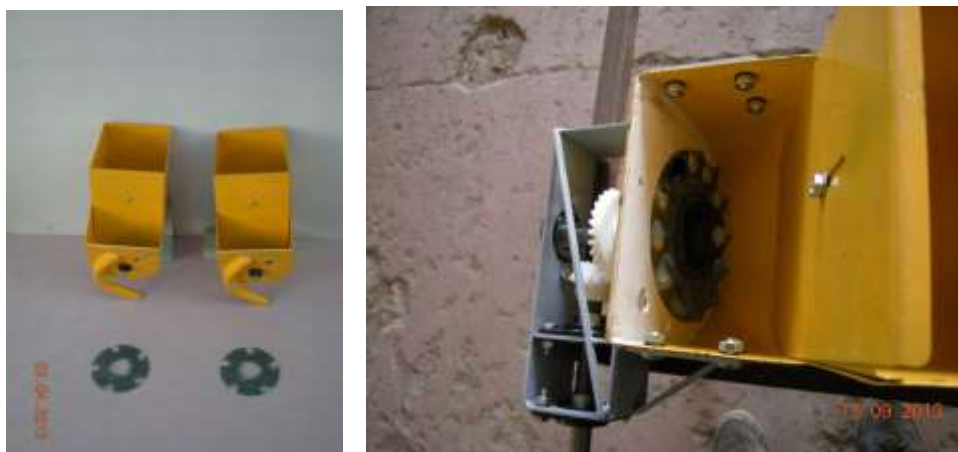
A basic inclined plate seed box and meter (left) and the assembled unit complete with drive gears (right)
