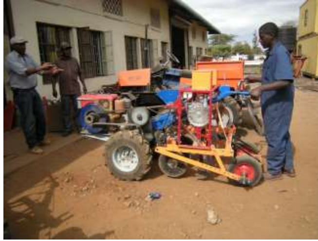
Completed seed drill (optional cutting coulter discs fitted)
