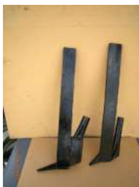
Tine with rake angle 30 degrees (left) and 55 degrees (right)
